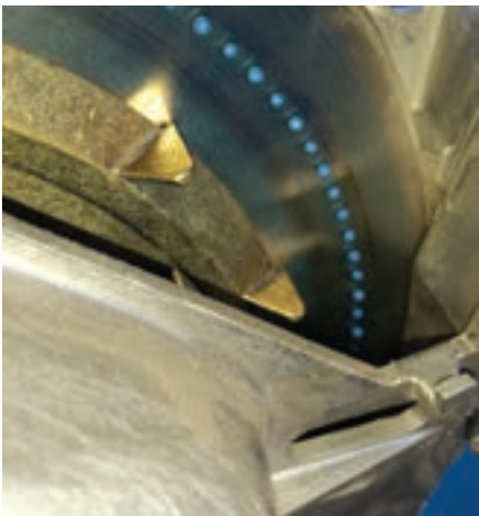
Canola seeds held in place by vacuum on the Monosem planter. PHOTO: FARMING SMARTER
