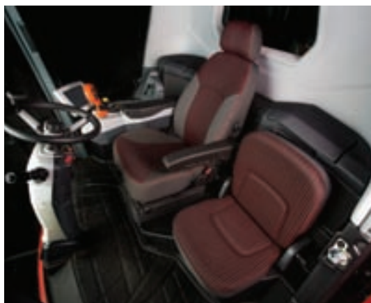
The combine cab is 30 per cent larger than its predecessor and has a more ergonomic control arrangement.
