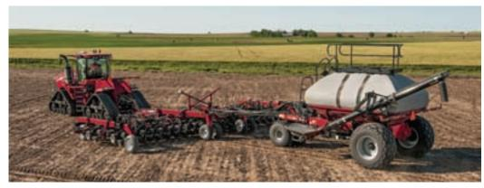
The latest technology in Case IH Precision Disk<sup>m</sup> air drills provides superior crop residue handling, seed placement and seed-to-soil contact for high-efficiency seeding in varying soils and terrains.
