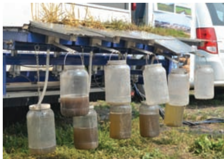
Run-off, collected in the top row of jars, is compared to the volume of water seeped through the earth after soil from five fields was exposed to the equivalent of a major rainfall event.
