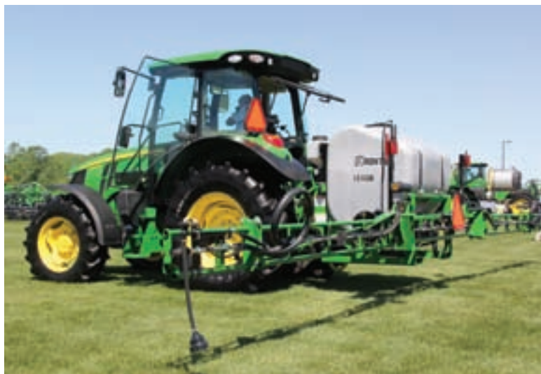
Sprayers: The LS11 line of three-point hitch sprayers are available with tank capacities of up to 300 U.S. gallons and 40-foot booms.
