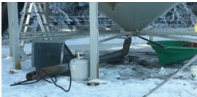
A frozen gate had to be melted with heat from a tiger torch focused through an old stovepipe.
