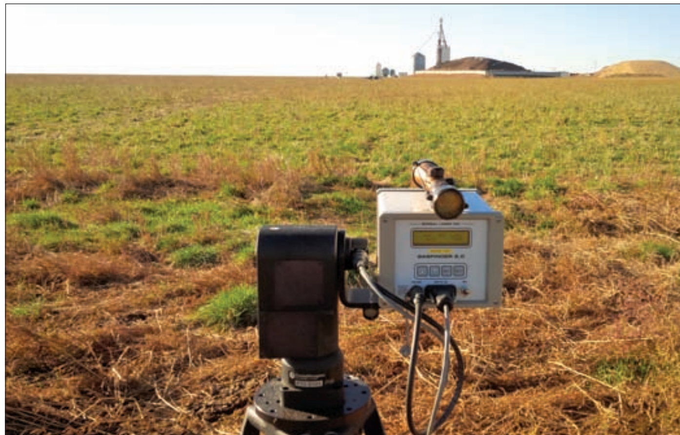
Using open-path lasers (pictured), federal research scientist Sean McGinn found between 50 to 60 per cent of nitrogen in a feedlot is lost to the atmosphere as ammonia. PHOTO: SUPPLIED
