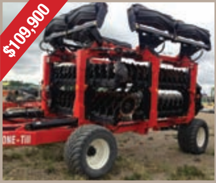
Pans 22", 22,000lbs, 10-15HP recommended, 12'6 transport height, 30'4 transport length, 12' transport width.
