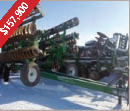
12.5m cutting width, 125KN Hub capacity, 100 discs, 4.8m transport width, 4m transport height, 15,800 kg
