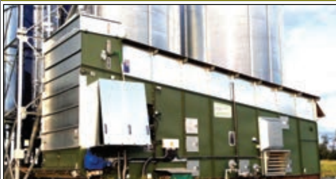
2014 - DF22 10' w x 40' L x 19' h 1000 bph on Cement
