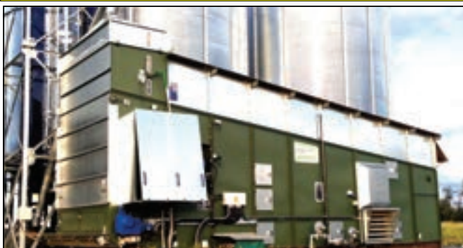
2014 - DF22 10' w x 40' L x 19' h 1000 bph on Cement
