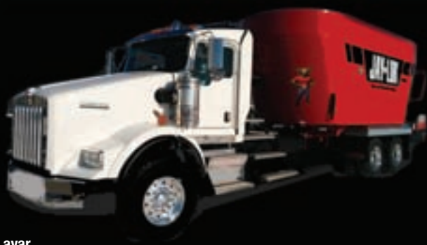
Jaylor 51250HD 5000 Series Twin Auger TMR Truck Mounted Mixer
