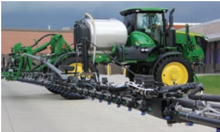
John Deere plans to introduce a carbon fibre sprayer boom to the North American market within the next couple of years.
