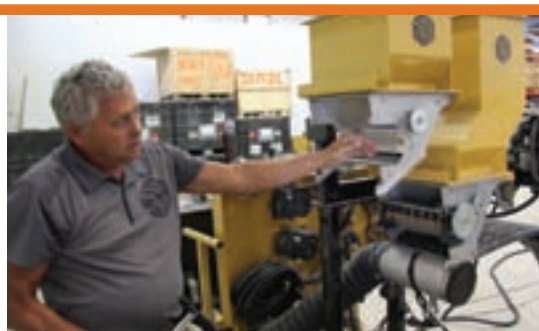
Company president Norbert Beaujot, explains the workings of a mock-up of a new metering system inside the R&D shop.
