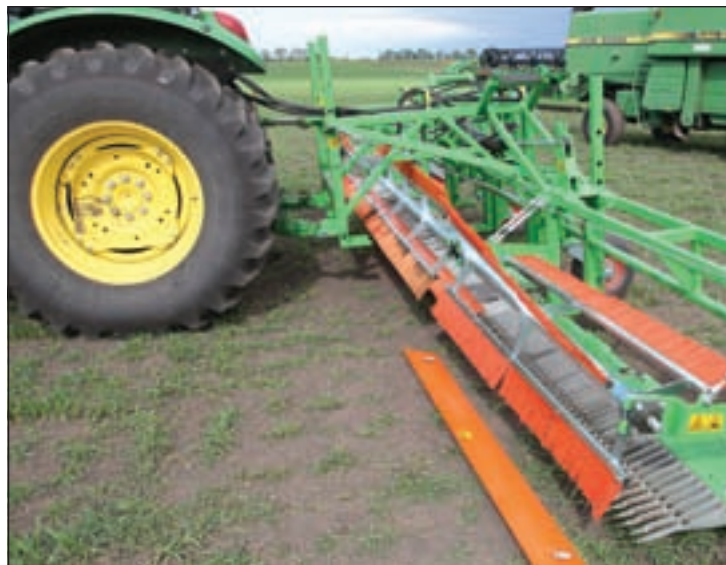
Cereal stems move unscathed through the CombCut's comb-like knives, while broadleaf weed stems are cropped close to the ground.
