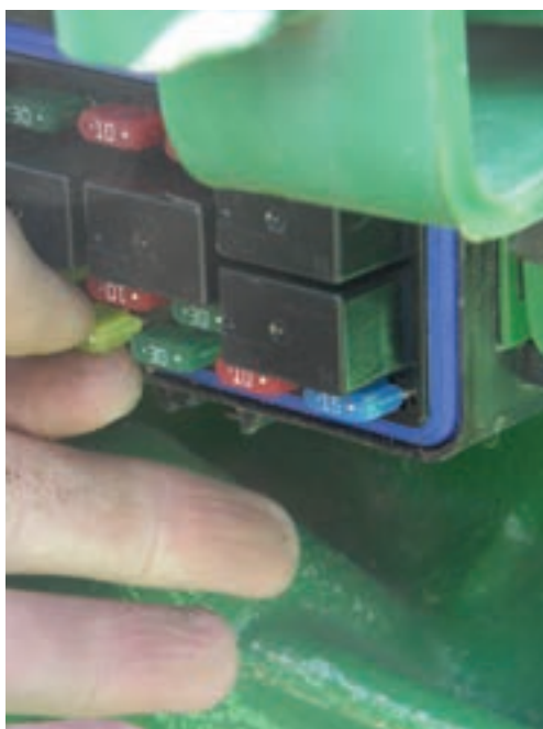
Removing one fuse at a time until the current flow stopped revealed which circuit had the faulty component.
