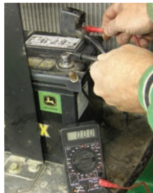
With the instrument panel gauge cluster disconnected, current flow fell to 0.0. That indicated the fault was in the gauge cluster and it will need to be replaced.
