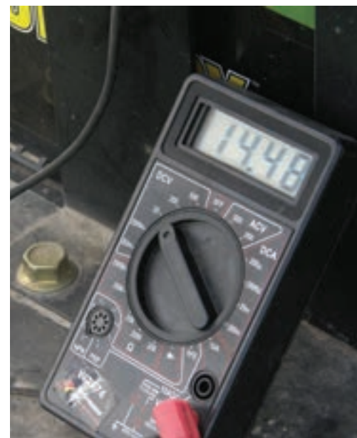
Before assuming a parasitic power drain was causing the battery to go dead, we checked the charging system with a multimeter. The multimeter reading of about 14.5 volts with the tractor engine running indicated the alternator was doing its job.
