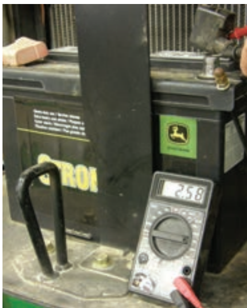
A fault in this tractor's electrical system was allowing a continuous 2.58 milliamp current to flow when engine and key were turned off, draining the battery within a couple of days.
