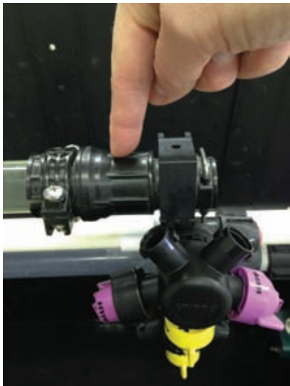
Hypro's Express boom end cap allows the last nozzle body to be mounted right at the end of the boom so there's no extra space for spray water to hide.
